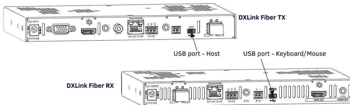
**FIG. 8** TX USB port – Host (top); RX USB port – Keyboard/Mouse (bottom)
