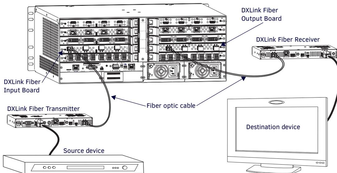
**FIG. 9** Endpoint Mode (Switcher) setup with Enova DGX 1600
