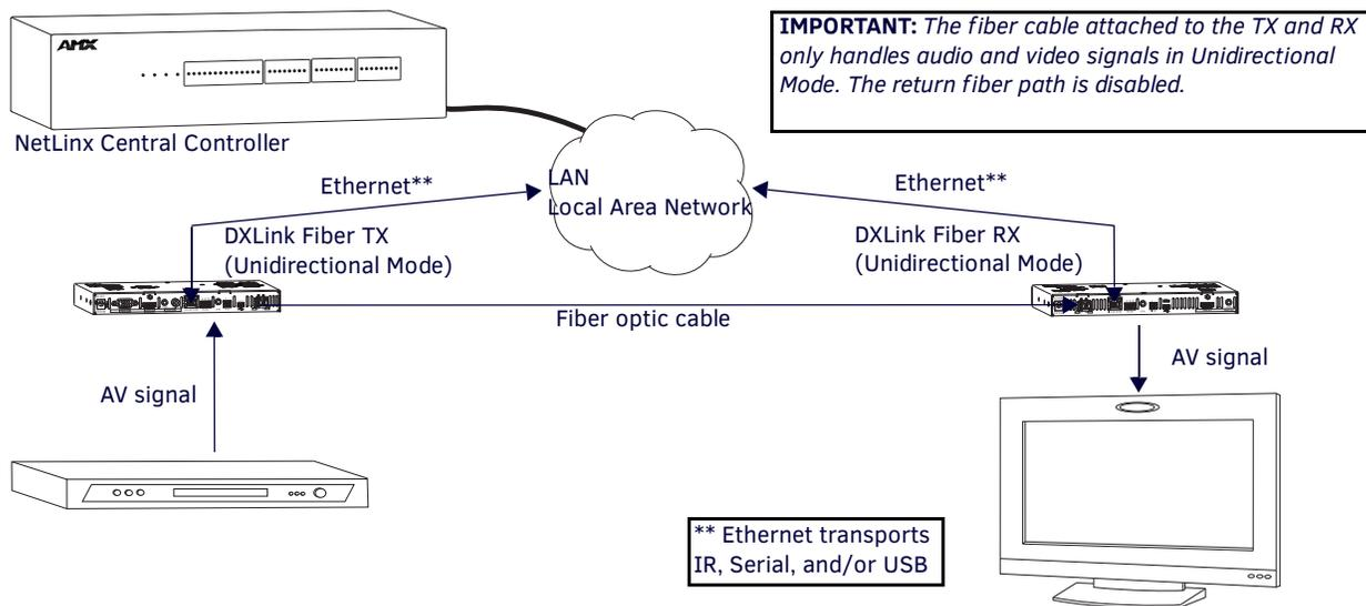
FIG. 24 Serial data transfer and IR flow control with hardware in Unidirectional Mode
