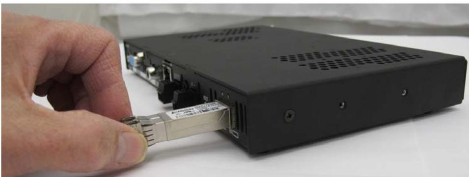
**FIG. 39** Insert transceiver into transceiver socket
