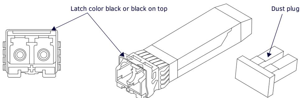
**FIG. 1** Multimode SFP+ fiber optic transceiver (model with black label on latch top shown)
