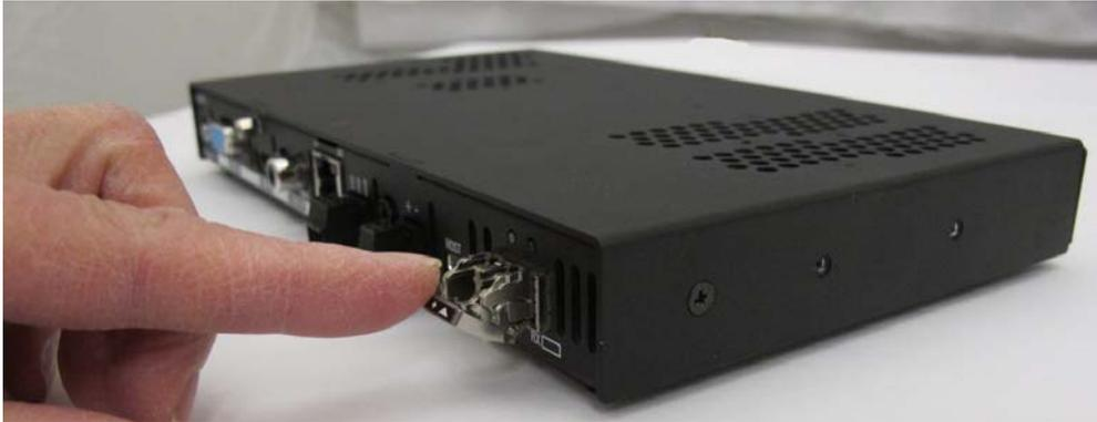
**FIG. 37** Flip transceiver latch out and down (DXLink Fiber Transmitter shown)
