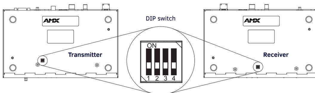
**FIG. 7** DIP switch location on DXLink Fiber units
