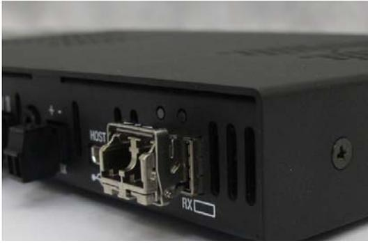
**FIG. 40** Transceiver latch in upright position
