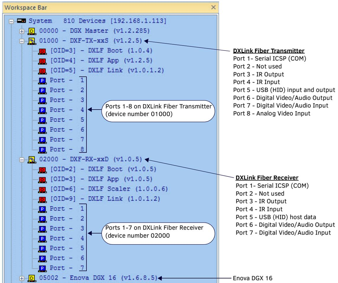
**FIG. 31** NetLinX Studio OnLine Tree - Ports 1-8 on DXLink Fiber Transmitter and Ports 1-7 on Receiver
