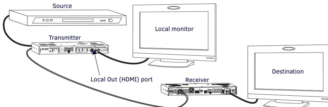
FIG. 28 Local Out port on front of TX sends source signal to local monitor
