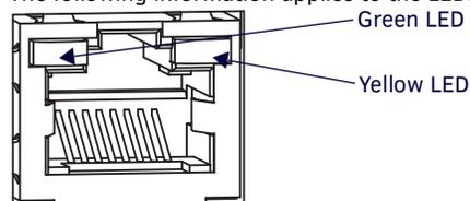
**FIG. 19** ICS LAN 10/100 connector LEDs on the DXLink Fiber units
