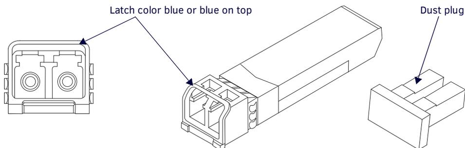
**FIG. 2** Single mode SFP+ fiber optic transceiver (model with blue latch shown)
