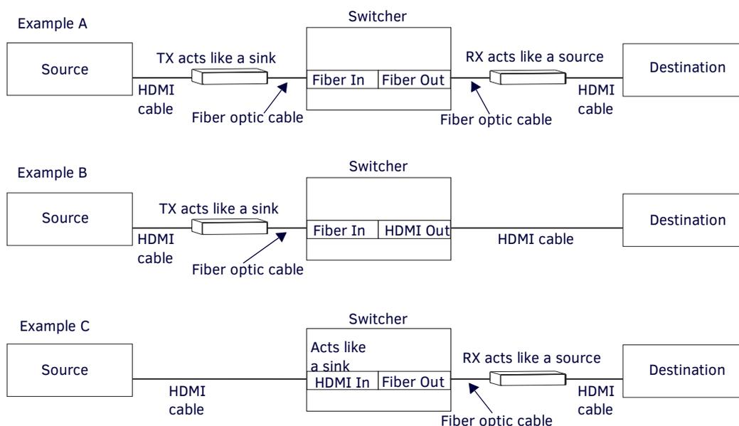
**Example A:** When a Receiver acts like a source, its key does not count. Source device sees 1 key (Transmitter).
