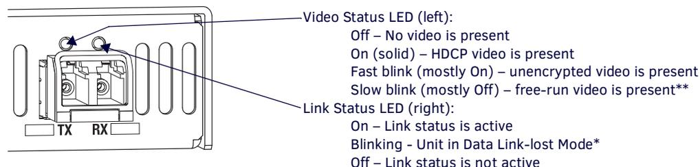
**FIG. 16** Fiber optic transceiver LEDs on Duplex hardware
