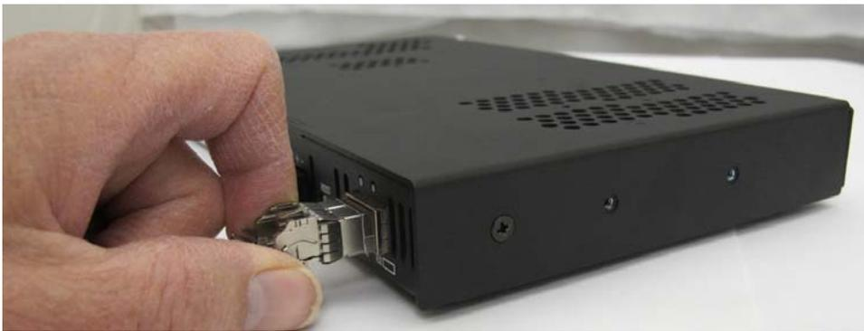
**FIG. 38** Pull transceiver free from transceiver socket
