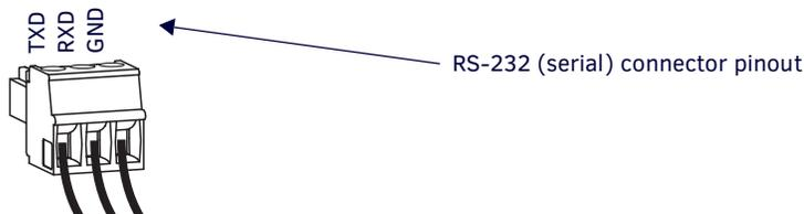
**FIG. 25** Wire RS-232 for serial data transfer
