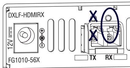
**FIG. 17** Fiber optic transceiver LEDs shown on TX (left) and RX (right)
