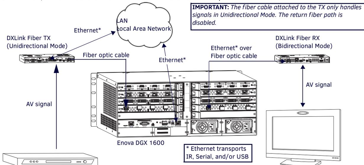
FIG. 23 Serial data transfer and IR flow control with TX in Unidirectional Mode and RX in Bidirectional Mode (Enova DGX 1600 shown)
