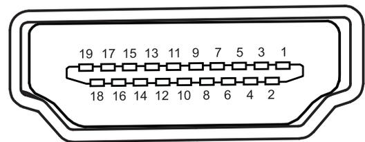
**FIG. 33** Pinout table and HDMI receptacle pins on DXLink Fiber unit
