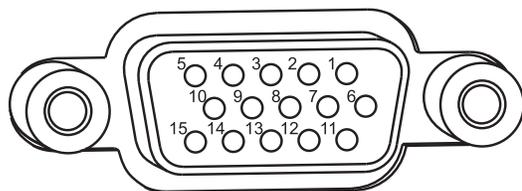
**FIG. 34** Pinout table and HD-15 receptacle pins on DXLink Fiber unit
