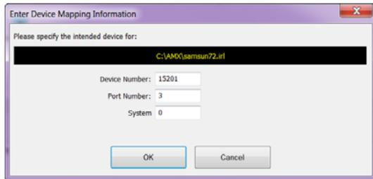
**NOTE:** IRL files must be sent to Port 3 (IR Device Port) on the Transmitter or Receiver.
