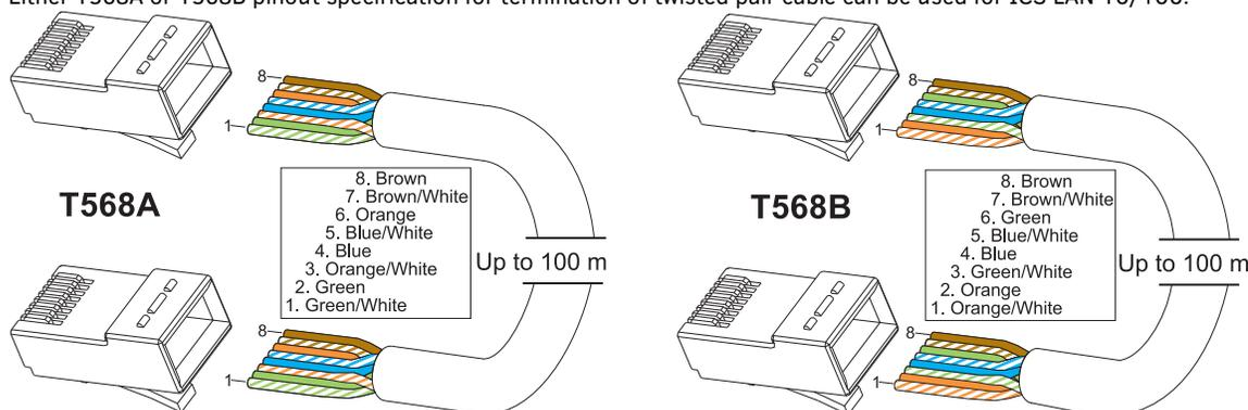
**FIG. 18** Twisted pair cable pinouts for Ethernet connectors
