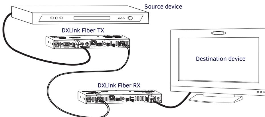
FIG. 12 Extender Mode (Standalone) system
