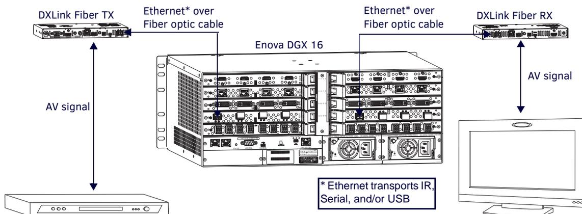
**FIG. 22** Serial data transfer and IR flow control with Duplex hardware in Bidirectional Mode
