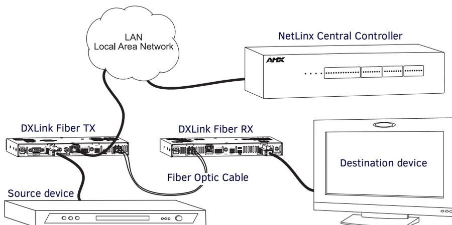
**FIG. 11** Endpoint Mode (Standalone) with NetLinX Central Controller
