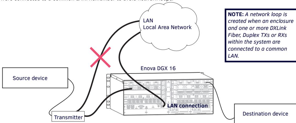
FIG. 13 Avoid network loops with DXLink Fiber, Duplex units in Bidirectional Mode
